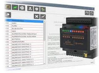
01 Negative 02 Analog Input 1 03 Analog Input 2 04 Analog Input 3 **05** Analog Input 4 **06** Positive 3,3VDC **07** Digital Input 1 08 Digital Input 2 09 Digital Input 3 **10** Digital Input 4 11 Digital Input 5 12 Digital Input 6 13 Power Supply **14** Power Supply 15 -**16** Relays common
