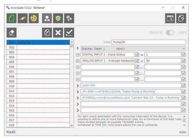
In this example the TRIGGER is Digital Input 1 and the CONDITIONS are a) It is activated (=1 closed) AND b) the 2<sup>nd</sup> CONDITION is that Analog Input1 is less that 30degC (attached NTC temperature probe) then the ACTIONS are performed to turn on Output1 AND send an SMS AND an EMAIL to confirm the pump is running (all in the one RULE).
